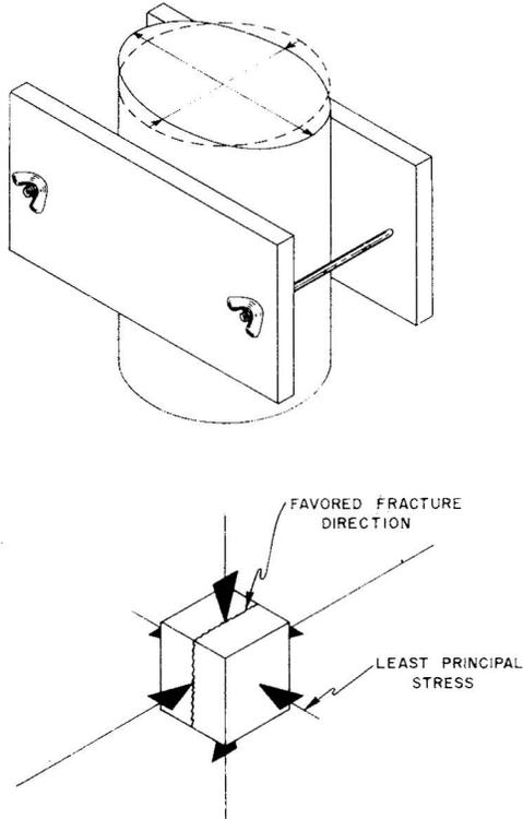
FIG. 21—EXPERIMENTAL ARRANGEMENT FOR PRODUCING THE LEAST STRESS IN A HORIZONTAL DIRECTION.
