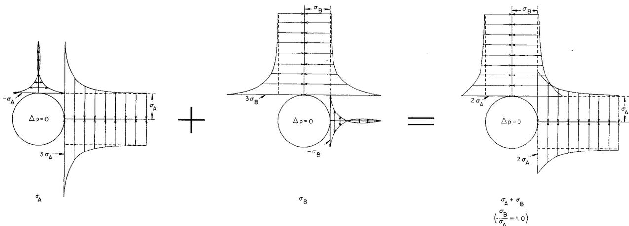
FIG. 13—SUPERPOSITION OF STRESS STATES ABOUT A WELLBORE DUE TO TWO HORIZONTAL PRINCIPAL STRESSES OF EQUAL MAGNITUDE.
