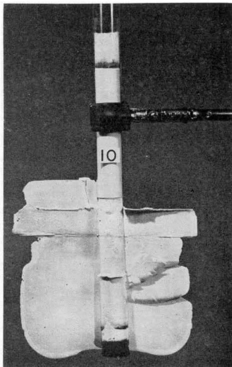
FIG. 25—VERTICAL FRACTURE IN STRATIFIED GELATIN.
