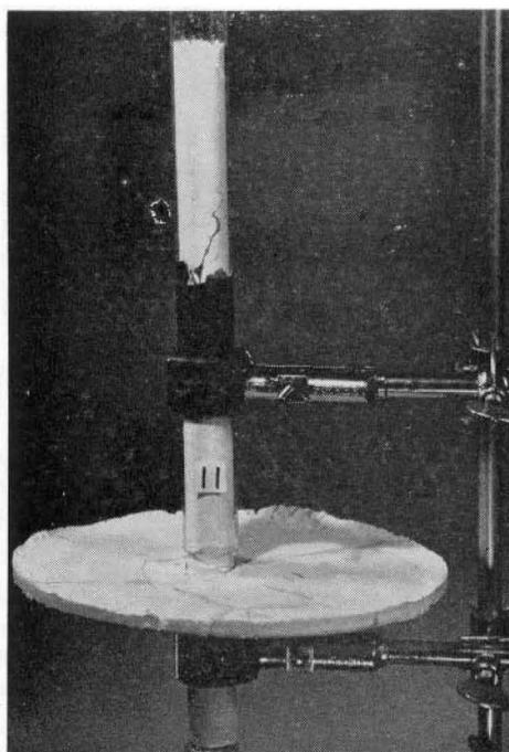
FIG. 26—HORIZONTAL FRACTURE IN STRATIFIED GELATIN.
