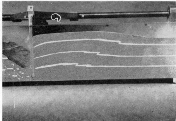
FIG. 3—SAND-BOX EXPERIMENT SHOWING THRUST FAULT.
