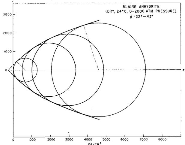
FIG. 12—MOHR ENVELOPES FOR BLAINE ANHYDRITE (MEASUREMENTS BY JOHN HANDIN).
