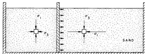
FIG. 4—SECTION SHOWING APPROXIMATE STRESS CONDITIONS IN SAND BOX.
