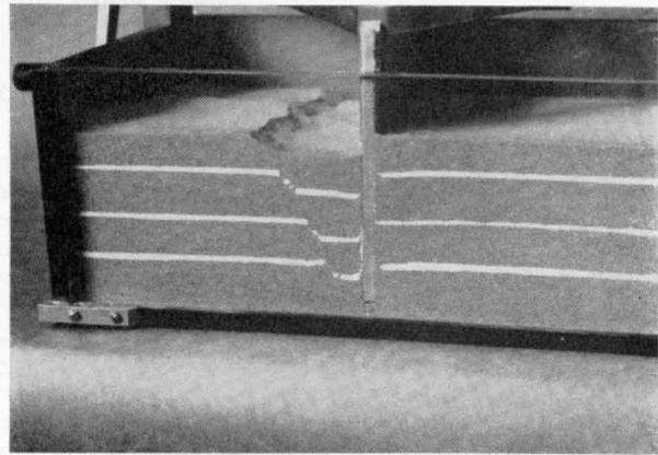
FIG. 2—SAND-BOX EXPERIMENT SHOWING NORMAL FAULT.
