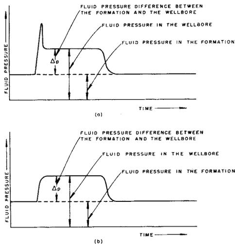
FIG. 18—IDEALIZED DIAGRAM OF TWO POSSIBLE TYPES OF PRESSURE BEHAVIOR DURING FRACTURE TREATMENT DEPENDING UPON VARIOUS UNDERGROUND CONDITIONS.
