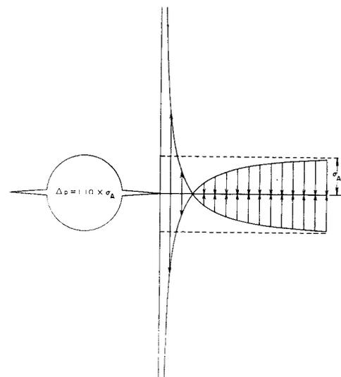
FIG. 17—STRESSES IN THE VICINITY OF A CRACK IN A STRESSED ELASTIC MATERIAL WHEN THE PRESSURE ACTING ON THE WALLS OF THE CRACK IS SLIGHTLY GREATER THAN THE STRESS WITHIN THE MATERIAL.
