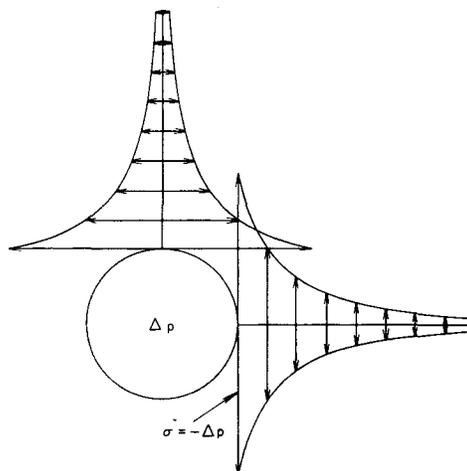
FIG. 15—STRESSES CAUSED BY A PRESSURE  $\Delta p$  WITHIN THE WELLBORE.
