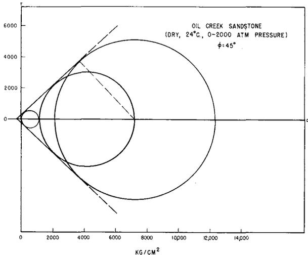
FIG. 11—MOHR ENVELOPES FOR OIL CREEK SANDSTONE (MEASUREMENTS BY JOHN HANDIN).
