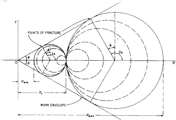
FIG. 9—MOHR DIAGRAM SHOWING THE POSSIBLE RANGE OF THE HORIZONTAL STRESS FOR A GIVEN VERTICAL STRESS  $\sigma_z$ . THE HORIZONTAL STRESS CAN HAVE ANY VALUE RANGING FROM APPROXIMATELY ONE-THIRD THE VERTICAL STRESS, CORRESPONDING TO NORMAL FAULTING, TO APPROXIMATELY THREE TIMES THE VERTICAL STRESS, CORRESPONDING TO REVERSE FAULTING.
