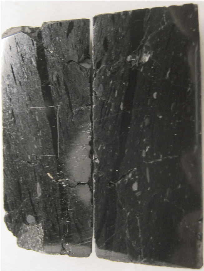
Fig. 1. A typical cylindrical sample's polished fracture surface.
