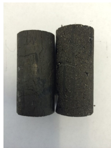
Fig. 2. Photograph of cylindrical Hazelton anthracite core samples.
