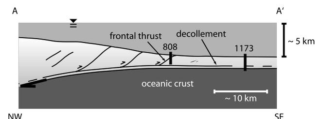
**Figure 5.** Schematic cross section of Nankai accretionary prism and ACORK locations. The décollement initiates between ODP Sites 808 and 1173. Though the ODP Site 808 borehole penetrates the décollement, the ACORK installation terminates above the décollement.
