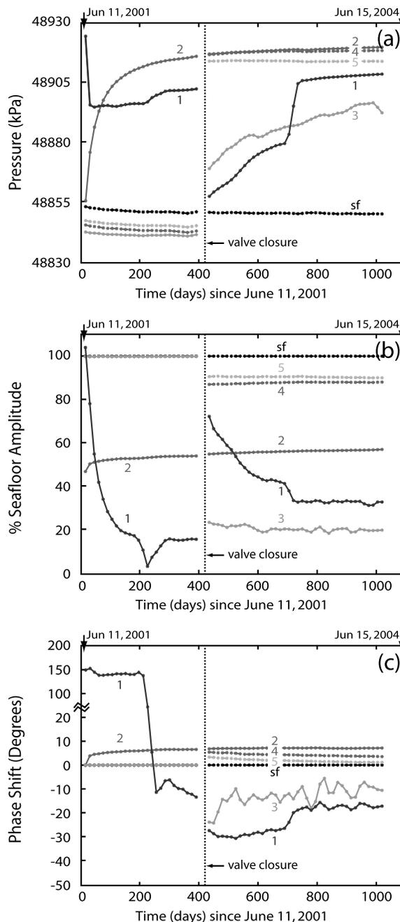
**Figure 12.** (a) Mean pressure versus time since installation at ODP Site 1173. (b) Amplitude response versus time for the  $M_2$  (semidiurnal) tidal signal. (c) Phase shift versus time for the  $M_2$  (semidiurnal) tidal signal. Open pump valves for screens 3, 4, and 5 were discovered and closed at approximately 400 days. Elevated fluid pressures, small amplitudes, and large phase shifts at screen 1 indicate that the bridge plug seals the inner casing and isolates screen 1 from the seafloor.
