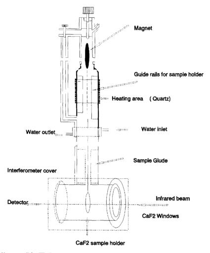
Fig. 1. Vacuum cell for FT-IR measurements. From Akhter et al., Appl. Spectrosc., 39(1) (1985) 143 [25].
