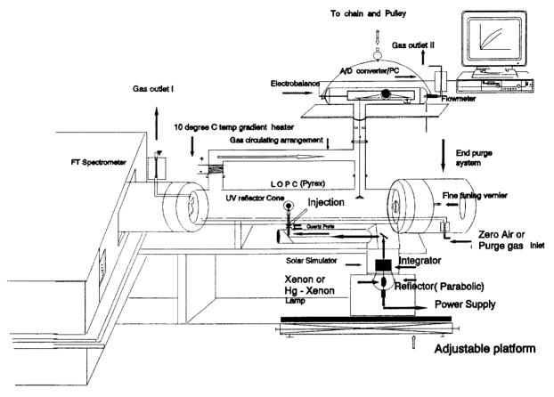
Fig. 2. Long optical path cell interfaced with FT spectrometer and electrobalance.
