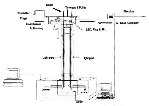
Fig. 31. Vertical LOPC interfaced with FT-IR spectrometer, electrobalance and 486PC.
