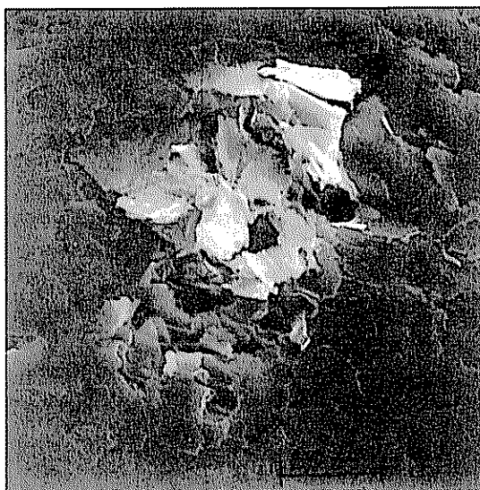
Fig. 7. The edge surface after its reaction with NiO in the presence of CO 2 (616 μm pressure) at 950°C for 1 hour. The pits formed in this case are shallower than those formed under similar conditions when the reaction was carried out in vacuum (cf. Fig. 6) and even when it was carried out for only 30 min (cf. Fig. 4).
