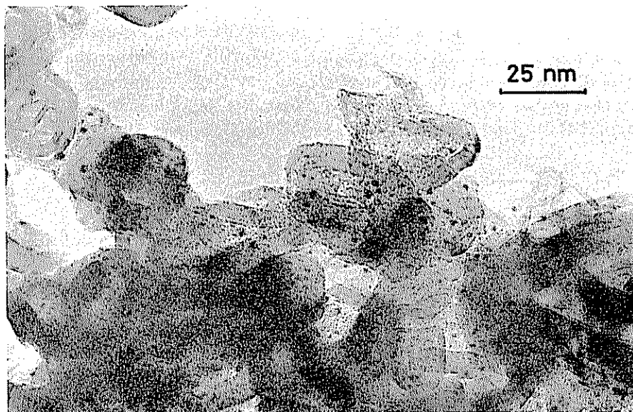
FIG. 2. Micrograph of platinum particles on activated carbon support following preparation at 773 K ( \times 800,000 ).
