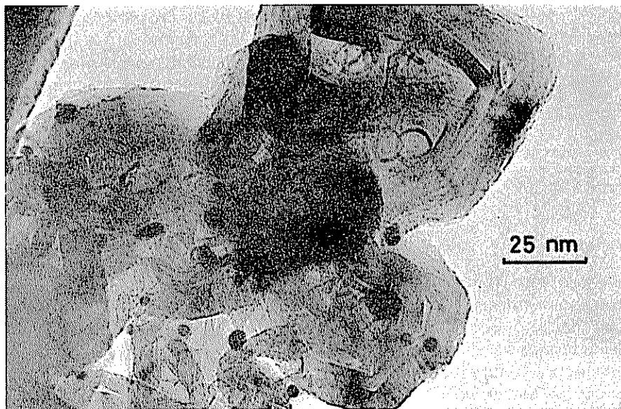
FIG. 1. Micrograph of platinum particles on unactivated carbon support following preparation at 773 K ( \times 800,000 ).
