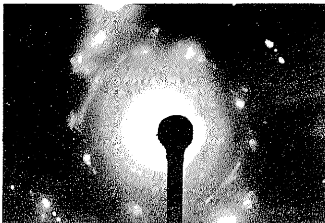
Figure 13. Selected-area electron diffraction pattern of the carbon shown in figure 12(c).
