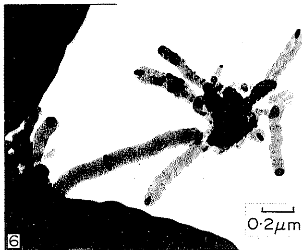
Fig. 6. Numerous filaments emanating from a central stem formed when iron is heated in methane at 900°C.
