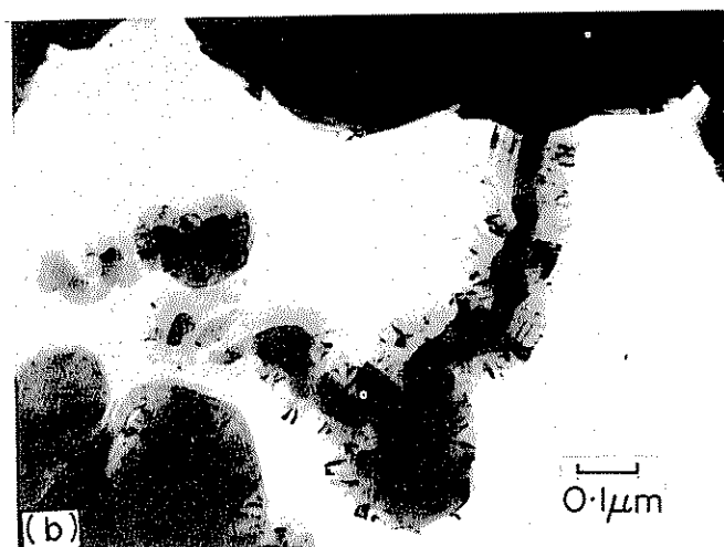
Fig. 4b. High resolution micrograph of filament formed when nickel is heated in methane at 900°C. Note numerous elongated electrondense particles along the core.
