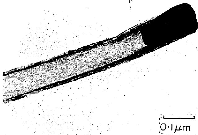
Fig. 1. Hollow filamentary growth, graphitic in nature, bearing an electron dense tip formed on exposure of stainless steel to commercial grade methane at 550°C.
