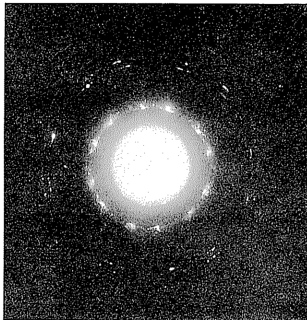
Fig. 8. Selected area diffraction pattern from a single graphite platelet deposited on (111) Ni
