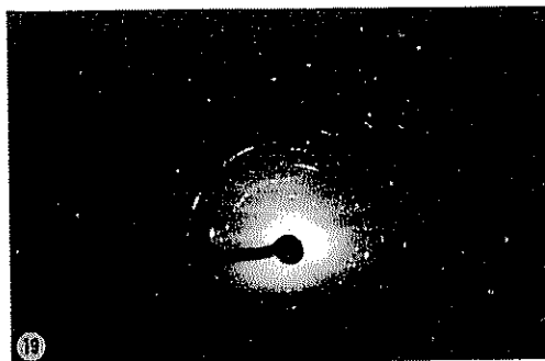
Fig. 19. Transmission electron diffraction pattern from a group of the whiskers shown in Fig. 18.
