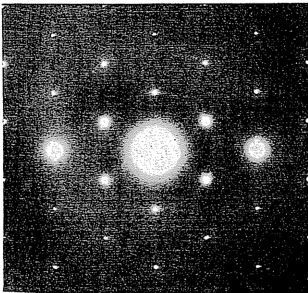
Fig. 18. Selected area electron diffraction pattern of graphite crystals (corresponding to Fig. 17) formed on Ni.
