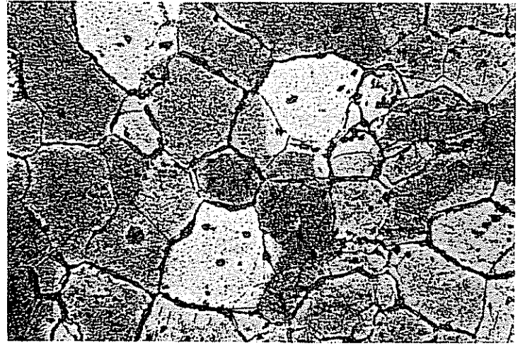
Fig. 1. Optical micrograph of surface of Pt foil after 20 min pyrolysis, showing decorated grain boundaries and variable nucleation density (154 \times ).
