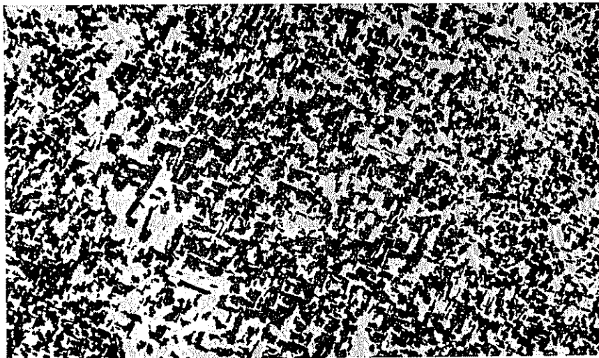
FIG. 7. Carbon film and WC resulting from interaction of evaporated carbon with W at 1000°C (11,000 \times ).
