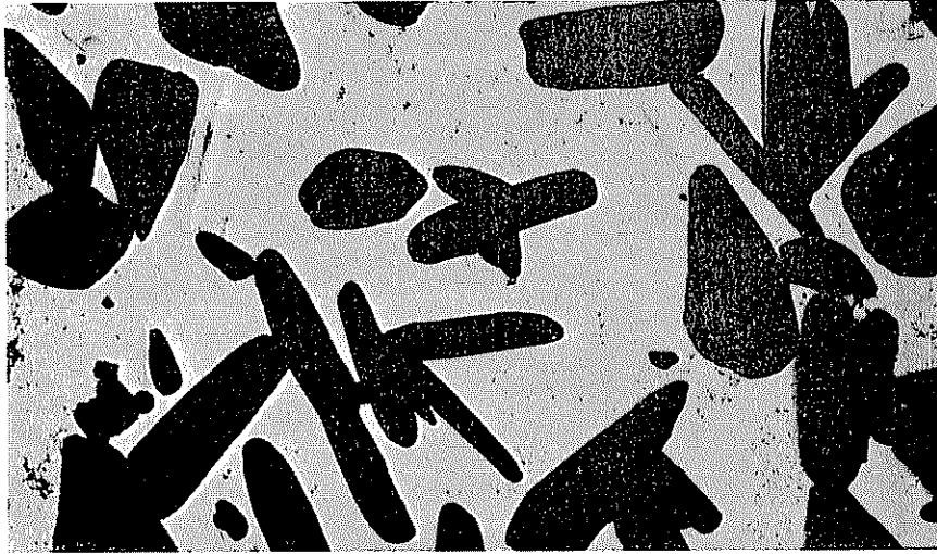
FIG. 9. Carbon film and TiC resulting from interaction of evaporated carbon with Ti at 1000°C (7500×).
