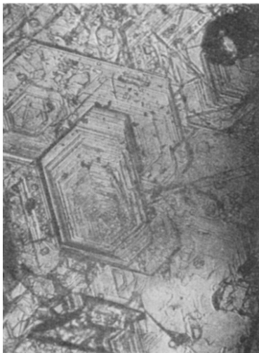
Fig. 3. Basal plane surface of purified kish showing large hexagonal stepped growth features. ( \times c. 200 )
