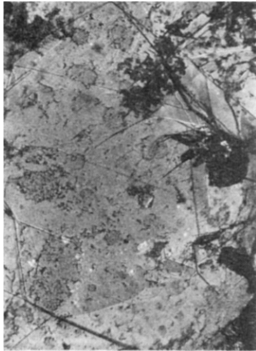
Fig. 2. Basal plane (000 \ell ) surface of kish purified in hydrochloric acid. Twin bands run parallel or intersect at 60°. ( \times c. 200 )
