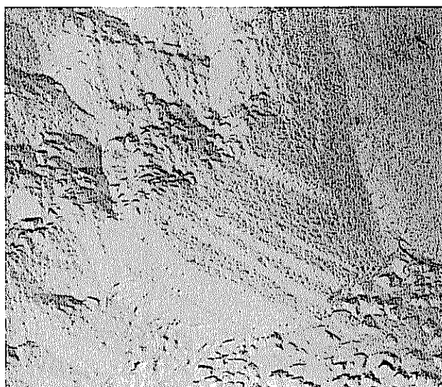
Fig. 5. Electron micrograph showing striations or steps formed on parts of the Ni surface under deposition conditions similar to those in Fig. 4. (7100X).
