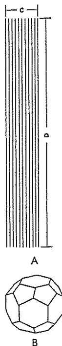
Fig. 7. Ideal structures of graphitized coke particles for the production of carbon bodies of low gas reactivity.
