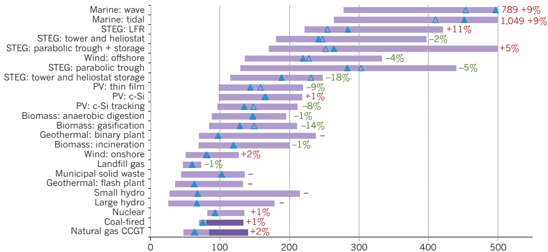
Figure 7 | Levelized cost of energy for quarter three, 2012. The analysis of cost in dollar per megawatt-hour is based on available data from projects in which investment or purchase contracts have been completed. To produce comparisons of levelized cost of energy at a global level, the analysis assumed a single corporate tax rate of 35%, an annual inflation of 2% and the equity investor internal rate of return of 10%. Quarter three central scenarios, filled triangles; quarter two central scenarios, open triangles. Adapted with permission from ref. 41.
