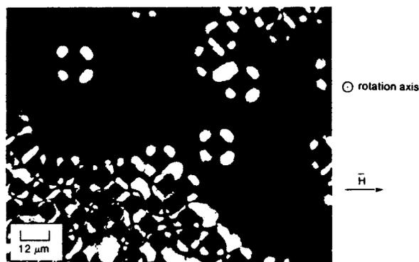
Figure 2. Micrograph of fiber bundle rotated in magnetic field perpendicular to bundle axis
