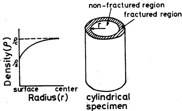
Fig. 1. A schematic of a cylindrical specimen with such a density gradient as shown in the left side. Fracture extends from the surface to the interior of the specimen.
