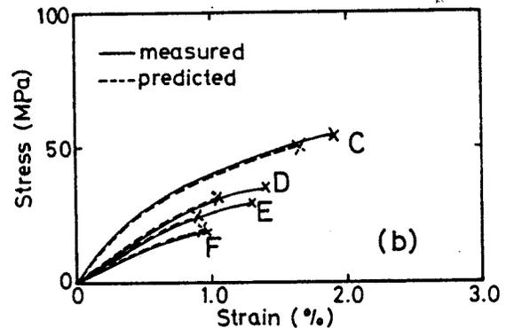
Figs. 2 (a), (b) Measured and predicted stress-strain curves. Cross marks indicate fractured. (a) Tensile tests (b) Compressive tests
