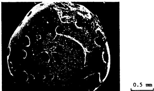
Figure 1. SEM micrograph of external fracture surface of shot coke.
