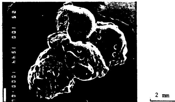
Figure 3. SEM micrograph of external surface of clustered shot coke.
