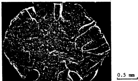
Figure 2. SEM micrograph of internal fracture surface of shot coke.
