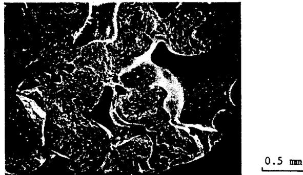
Figure 4. SEM micrograph of internal (fracture) surface of sponge coke.
