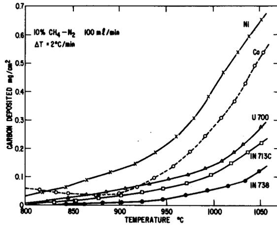
Fig. 1 Pyrolytic carbon formation on metals and alloys from  $10\% \text{CH}_4\text{-N}_2$ . Weight deposited vs. temperature.
