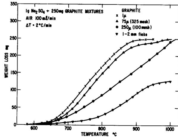
Fig. 2 Burnoff of graphite in air from  $\text{Na}_2\text{SO}_4$ -graphite mixtures. Effect of graphite particle size.
