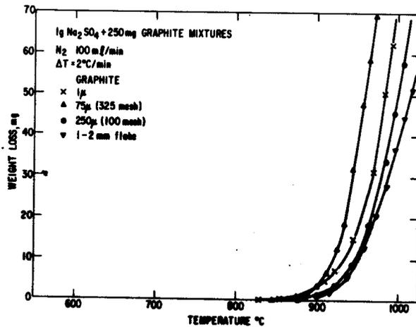
Fig. 3 Reduction of  $\text{Na}_2\text{SO}_4$  by graphite as a function of temperature and graphite particle size.
