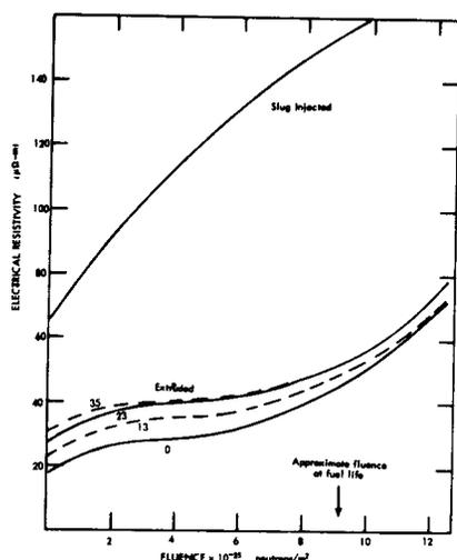
Fig. 3. The Room Temperature  $\rho$  of Extruded and Slug-Injected Fuel Elements Versus Neutron Fluence.
