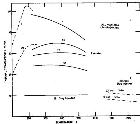
Fig. 1. The  $\lambda$  of Unirradiated Simulated-Fuel Elements versus  $T$ . The two low  $T$  curves were obtained on extruded elements with a different matrix.
