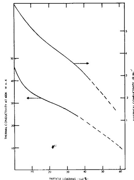
Fig. 2. The  $\lambda$  (400 K) and  $\sigma$  (300 K) of Unirradiated Simulated-Fuel Elements Versus Volume Percent Loading.
