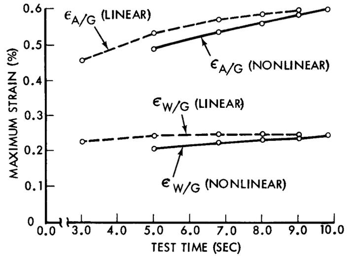
Figure 2. Maximum Across Grain and With Grain Strains Versus Test Time
