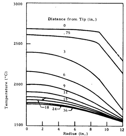
Figure 4. Temperature vs. radius at different distances from tip for a 24 in. diameter graphite electrode. Furnace wall temperature = 1500°C. Effective steel bath temperature = 2700°C. Current = 60 Kamp.
