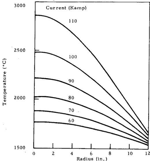
Figure 2. Temperature vs. radius for a 24 in. diameter graphite electrode conducting different currents. Furnace wall temperature = 1500°C.
