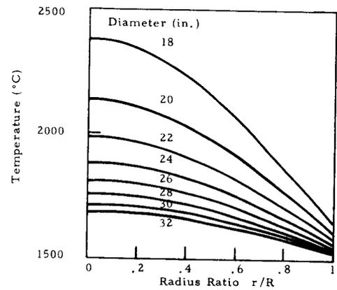
Figure 3. Temperature vs. normalized radius for graphite electrodes of different diameters. Furnace wall temperature = 1500°C. Current = 70 Kamp.
