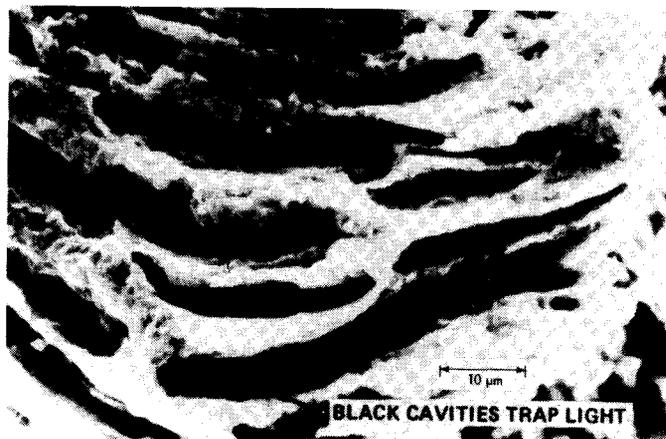
Fig. 2: Selective Absorbing Surfaces May be Formed by Controlling the Surface Morphology
