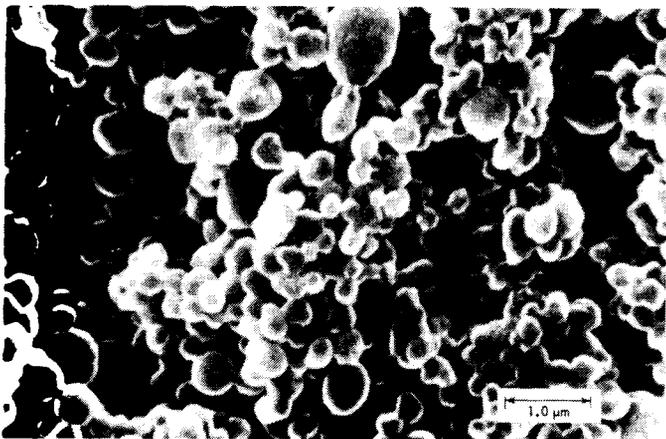
Fig. 1: The Heat-Treated, Thermax/Acrylic Coatings Contain Small, Spherical Particles
