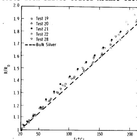
Fig. 2 - Resistance ratio for silver-plated fibers in helium.
