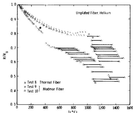
Fig. 1 - Resistance ratio for unplated fibers in helium.
