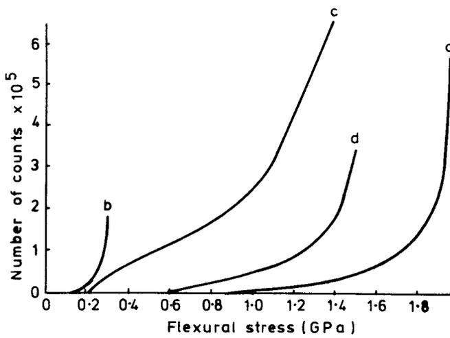
Figure 1 Acoustic emission responses of (a) green, (b) carbonised, (c) isothermal CVD and (d) thermal gradient CVD carbon-carbon composites
