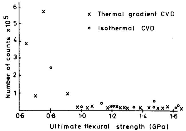
Figure 3 Relationship between the ultimate flexural strength and the acoustic emission monitored during flexural cycling between 0 and 0.4 GPa
