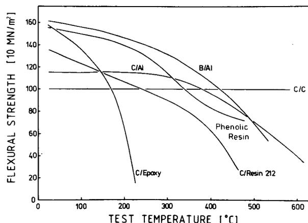
**Fig.2: Flexural strength of unidirectionally fiber reinforced composites as function of test temperature**
