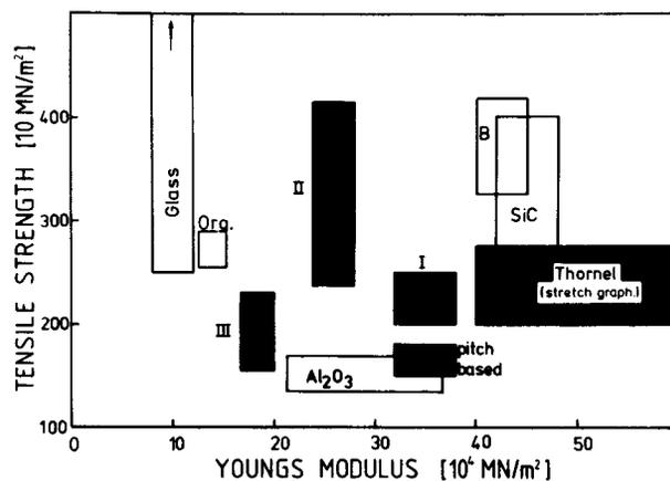
**Fig.1: Tensile strength and YOUNG's modulus of high performance fibre materials**
