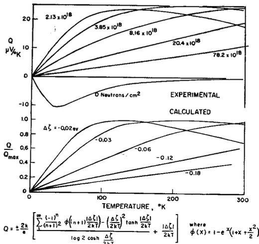
FIG. 3. The thermoelectric power vs temperature for differing neutron exposures.
