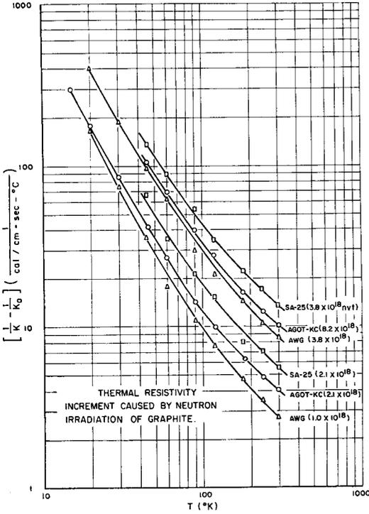
FIG. 18. Thermal resistivity change caused by neutron irradiation.
