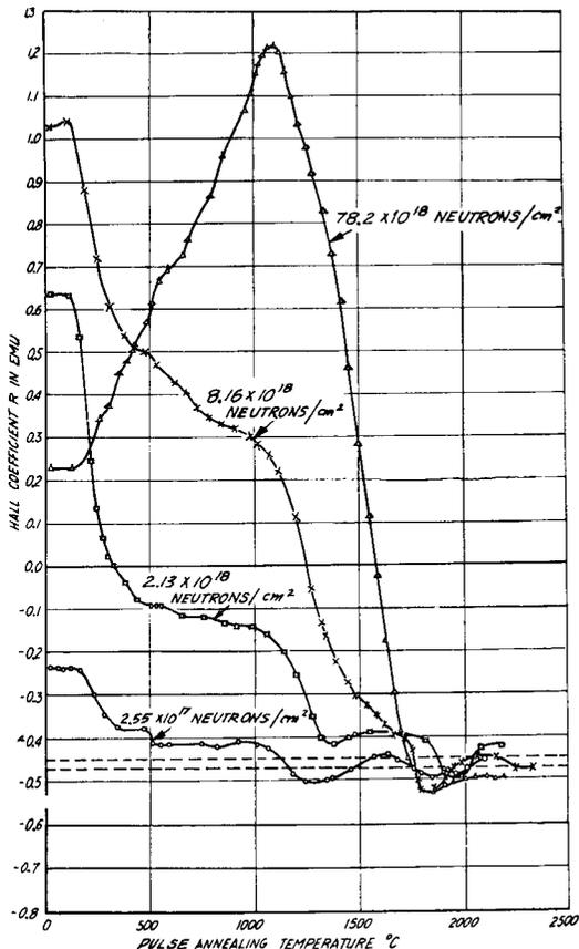
FIG. 11. Pulse-annealing spectrum of the Hall coefficient.
