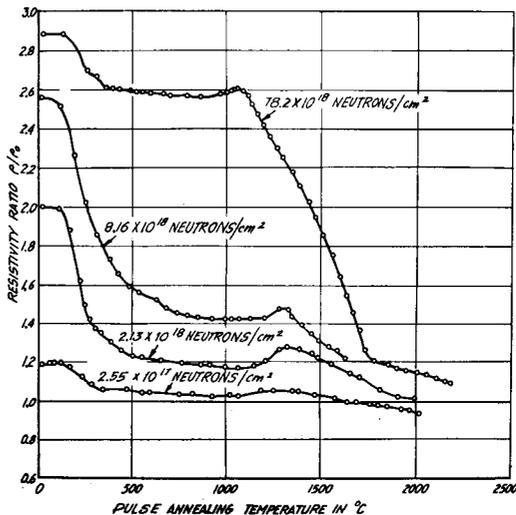
FIG. 14. Pulse-annealing spectrum of the electrical resistivity.
