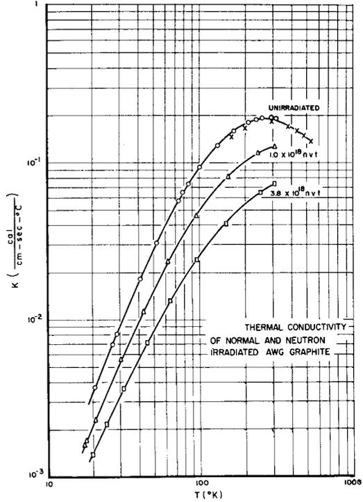
FIG. 17. Thermal conductivity of neutron-irradiated AWG graphite.
