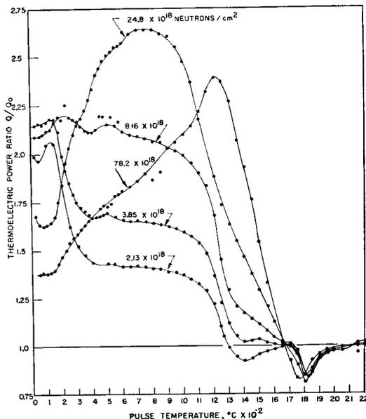
FIG. 12. Pulse-annealing spectrum of the thermoelectric power.
