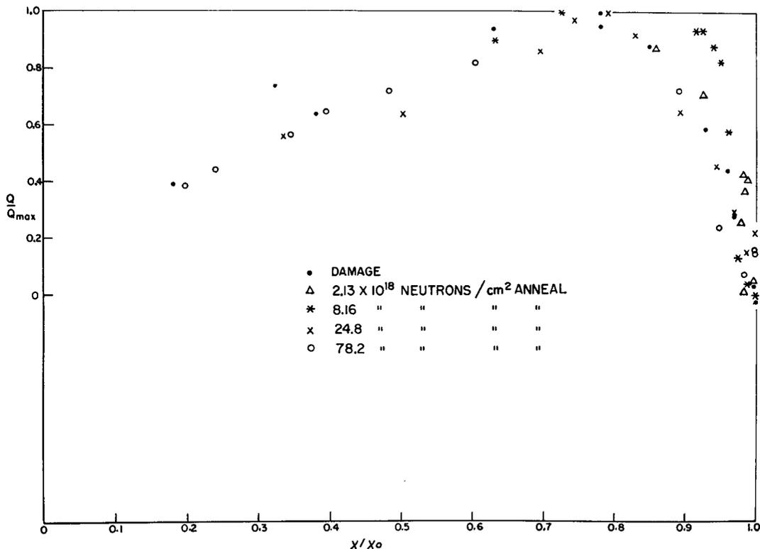
FIG. 10. Correlation of changes of thermoelectric power with susceptibility
