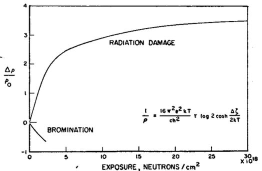
FIG. 6. Electrical resistivity change with neutron exposure and bromination.
