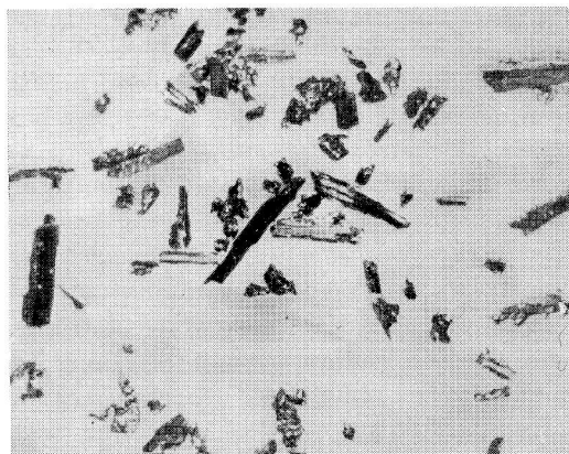
FIG. 4. Typical shapes of particles obtained by grinding a section of calcined Kendall coke with a strong needle structure. Magnification \times 20 .
