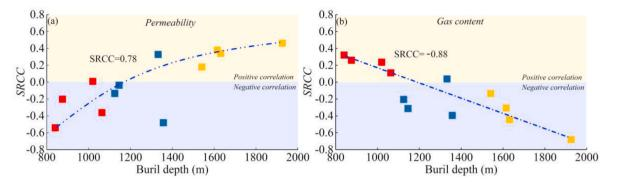
Fig. 7. Variation of SRCCs with burial depth for the various physical parameters defining the reservoir.
