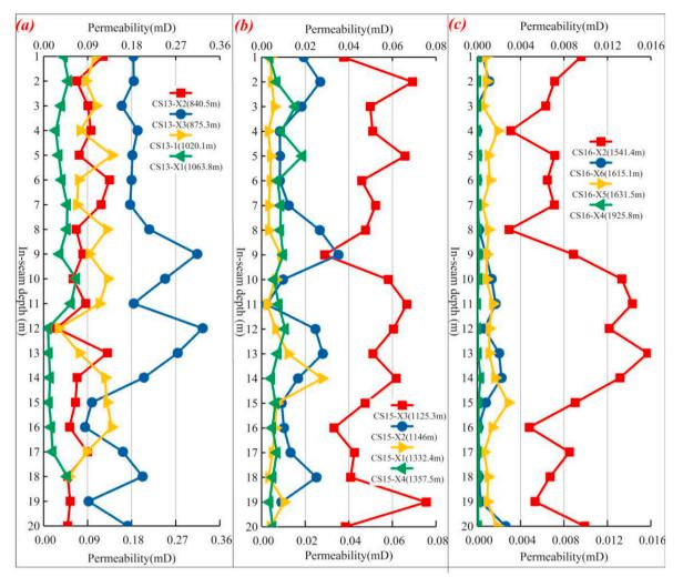
Fig. 4. Vertical heterogeneity in permeability of SDUT CBM reservoirs with in-seam depth, recovered from well.
