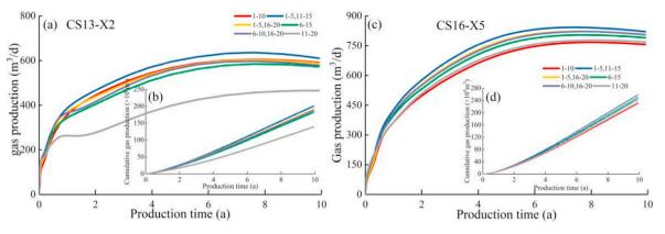
Fig. 16. Gas production rates for different combinations of perforation configuration.
