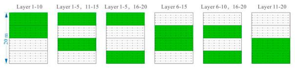
Fig. 15. Schematic diagram of the locations of perforations within SDUT CBM reservoirs.
