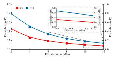
Fig. 9. Permeability and effective stress distribution recovered from reservoir samples buried at a depth of 650 m in the study block.
