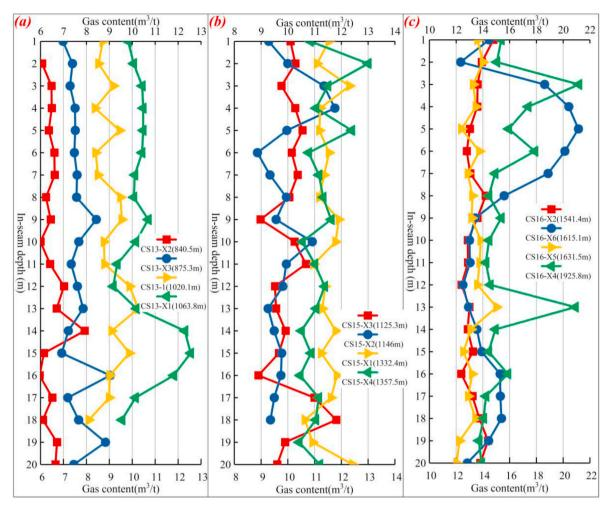
Fig. 5. Vertical heterogeneity in gas content of SDUT CBM reservoirs with in-seam depth, recovered from well logs.
