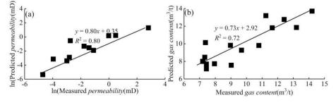
Fig. 3. Correspondence between well logging inversion data and measured data.
