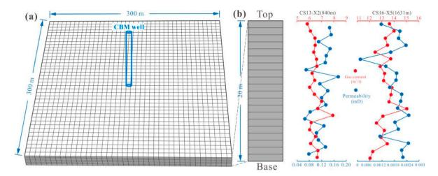
Fig. 13. Grid for numerical simulation (a) and vertical distribution of gas content and permeability of SDUT CBM reservoirs (b) gas contents and permeability across the seam.
