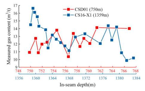
Fig. 6. Vertical heterogeneity of measured gas content of SDUT CBM reservoirs with in-seam depth, as a function of burial depth.
