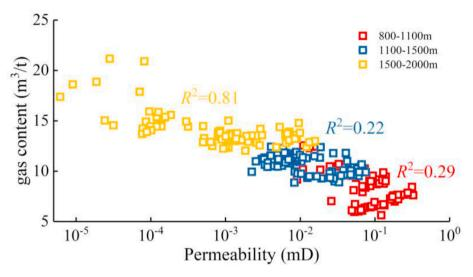
Fig. 8. Distribution of permeability and gas content in different burial depth range.
