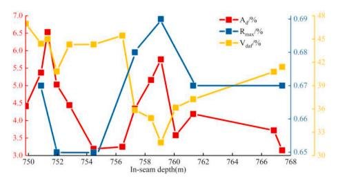
Fig. 10. Measured ash yield, vitrinite reflectance and volatile yield of SDUT CBM reservoirs in well CSD01.
