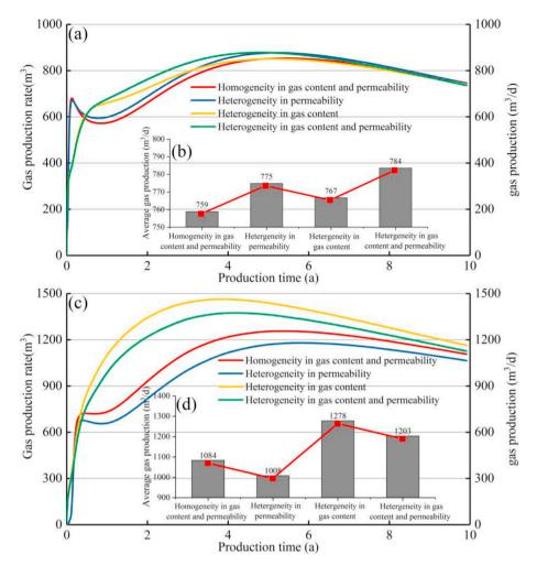
Fig. 14. Gas production profile and average daily gas production with a heterogeneous distribution of permeability and gas content of SDUT CBM reservoirs with depth.
