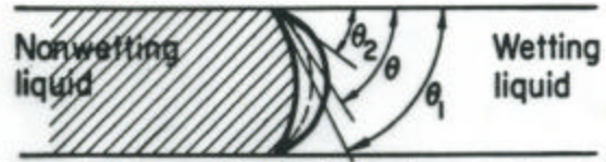
FIG. 9.2.8. Contact angle ( \theta ) in a capillary tube in a stationary state, in a displacement of a nonwetting liquid by a wetting one ( \theta_1 ) and in a displacement of a wetting liquid by a nonwetting one ( \theta_2 ).
