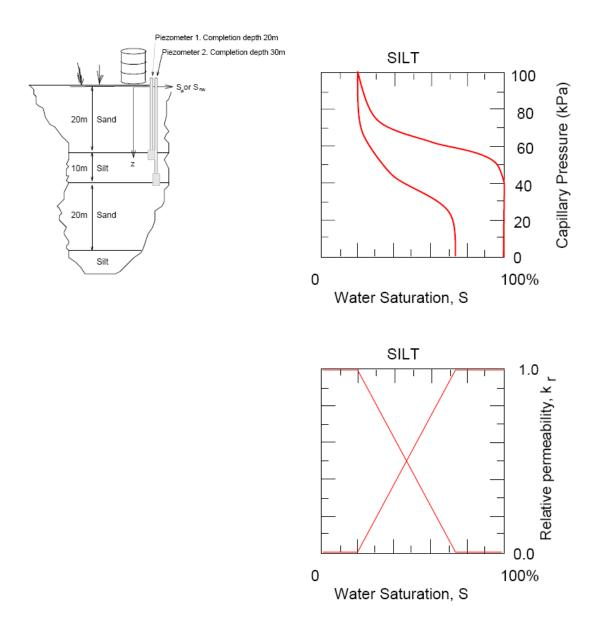
3. Evaluate the effective water and TCE saturations at the locations of each of the piezometers. Explain your rationale for choice of drainage or imbibition curves.
