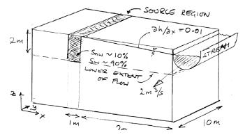
A surface spill of gasoline has penetrated into the subsurface. It previously rested on the groundwater table, which has fallen and subsequently risen, to smear it as shown. The floating free-product has been removed, and the smeared zone is below the water table and at a residual saturation of 90% water and 10% LNAPL.
