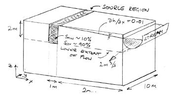
A surface spill of gasoline has penetrated into the subsurface. It previously rested on the groundwater table, which has fallen and subsequently risen, to smear it as shown. The floating free-product has been removed, and the smeared zone is below the water table and at a residual saturation of 90% water and 10% LNAPL.
