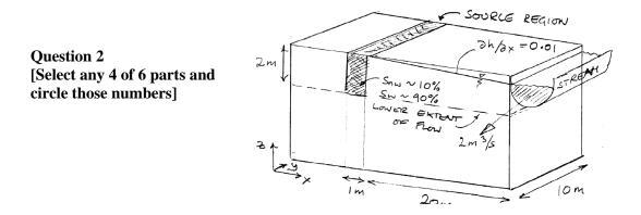
A surface spill of gasoline has penetrated into the subsurface. It previously rested on the groundwater table, which has fallen and subsequently risen, to smear it as shown. The floating free-product has been removed, and the smeared zone is below the water table and at a residual saturation of 90% water and 10% LNAPL.
