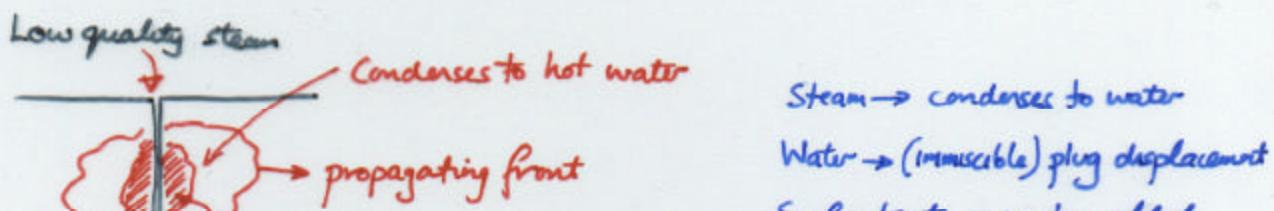
$$k_{rw} \uparrow \text{ by hot water due to viscosity} \\ \mu \propto \frac{1}{Temp} \propto \frac{1}{\text{Kelvin}}$$
