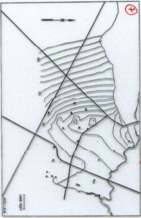
Figure 5.14. Water-table contours for RSC2 pumping 10 days from each well at "F" and injecting 2 mgm into each well at "T" (after Gray and Hoffman, 1983).
