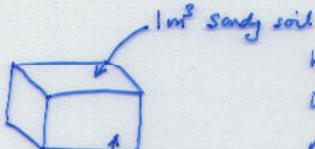
$$\left. \begin{array}{l} K = 10^{-3} \text{ cm/s} \\ i = 0.01 \\ n_e = 0.3 \end{array} \right\} V^a = \frac{Ki}{n} = \frac{10^{-3} \cdot 0.01}{0.3} = 3 \cdot 10^{-5} \text{ cm/s} = 3 \text{ cm/d} = .03 \text{ m/d}$$
