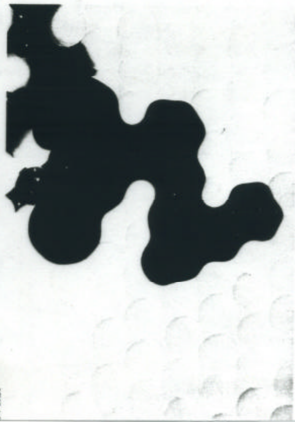
Figure XVI.a. Beads initially moist; diameter range = 0.85 - 1.23 mm. PER then dripped in from above. The PER accumulated as a sheath around a zone of high water content.
