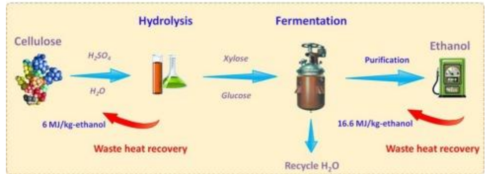
Energy-saving cellulose ethanol production process by heat integration
