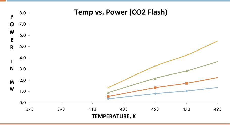
Flash power plants are favorable only above 473 K; whereas, the CO2 flash plant is comparable for net power generated with basic binary power plant and dual pressure binary power plant
