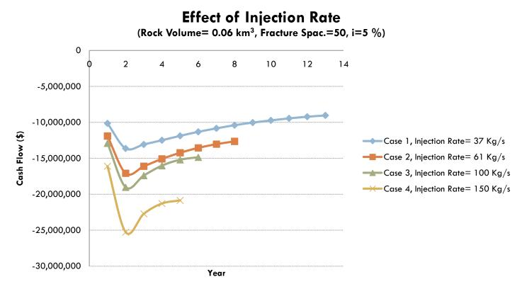
In higher injection rate case, project lifetime would decrease. Also, we have to invest more capital cost for power plant and pumping. HIGH INJECTION RATE IS NOT NECESSARILY BETTER
