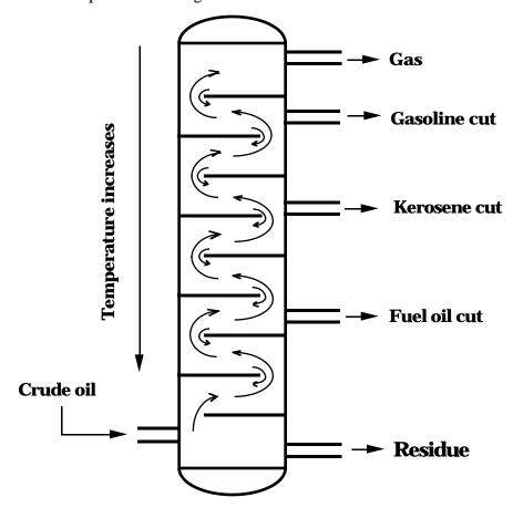
**FIGURE 8-13.** Schematic representation of a distillation tower.
