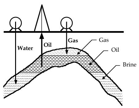
**FIGURE 8-9.** Enhanced oil recovery techniques: secondary recovery.
