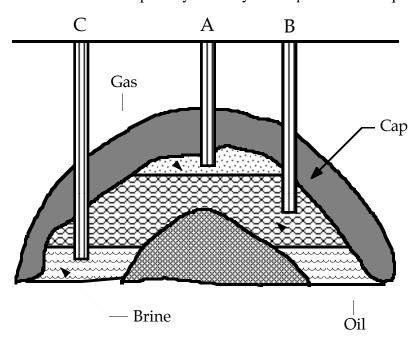
**FIGURE 8-7.** Selection of a site for petroleum drilling.
