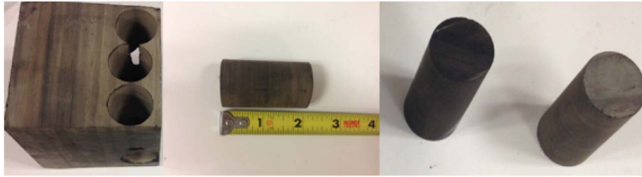
Fig. 1 Green River shale block and samples drilled parallel and perpendicular to the bedding plane
