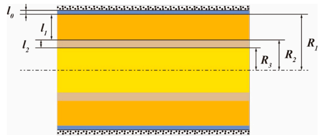
Fig. 1. Axisymmetric multiphase flow within a parallel-sided capillary. R_1 is the radius of the total flowing section. R_2 is the radius of the gas area (including the transition zone and bulk gas zone). In addition, l_0 , l_1 , and l_2 represent the thickness of the adsorbed water, bulk oil zone, and oil–gas transition.
