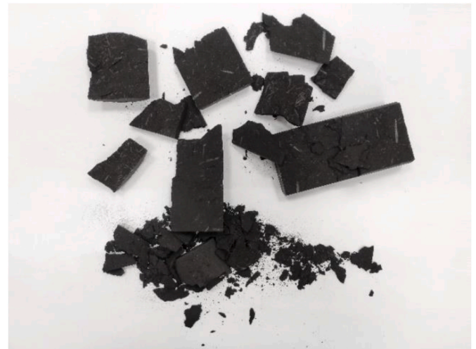
Fig. 3. Effects on shale samples of continuous microwave treatment.
