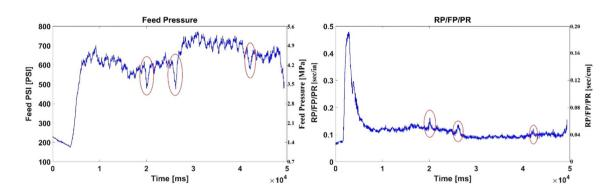
Fig. 11 Plot of feed pressure data and RP/FP/PR data for drilling in sample with inclined joints
