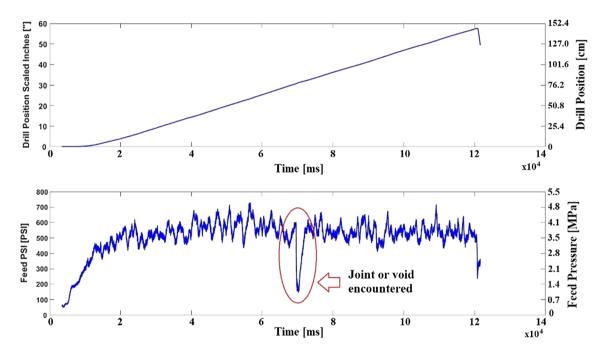
Fig. 5 Drill bit position and feed pressure (thrust) data
