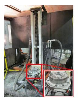
Fig. 3 J.H. Fletcher & Co. drill control unit. (Reproduced with permission from Bahrampour et al. 2015)
