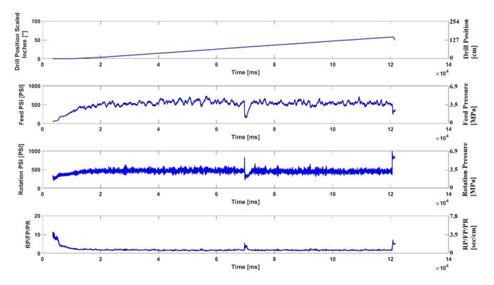
Fig. 7 RP/FP/PR, feed pressure and rotation pressure associated with drill bit position
