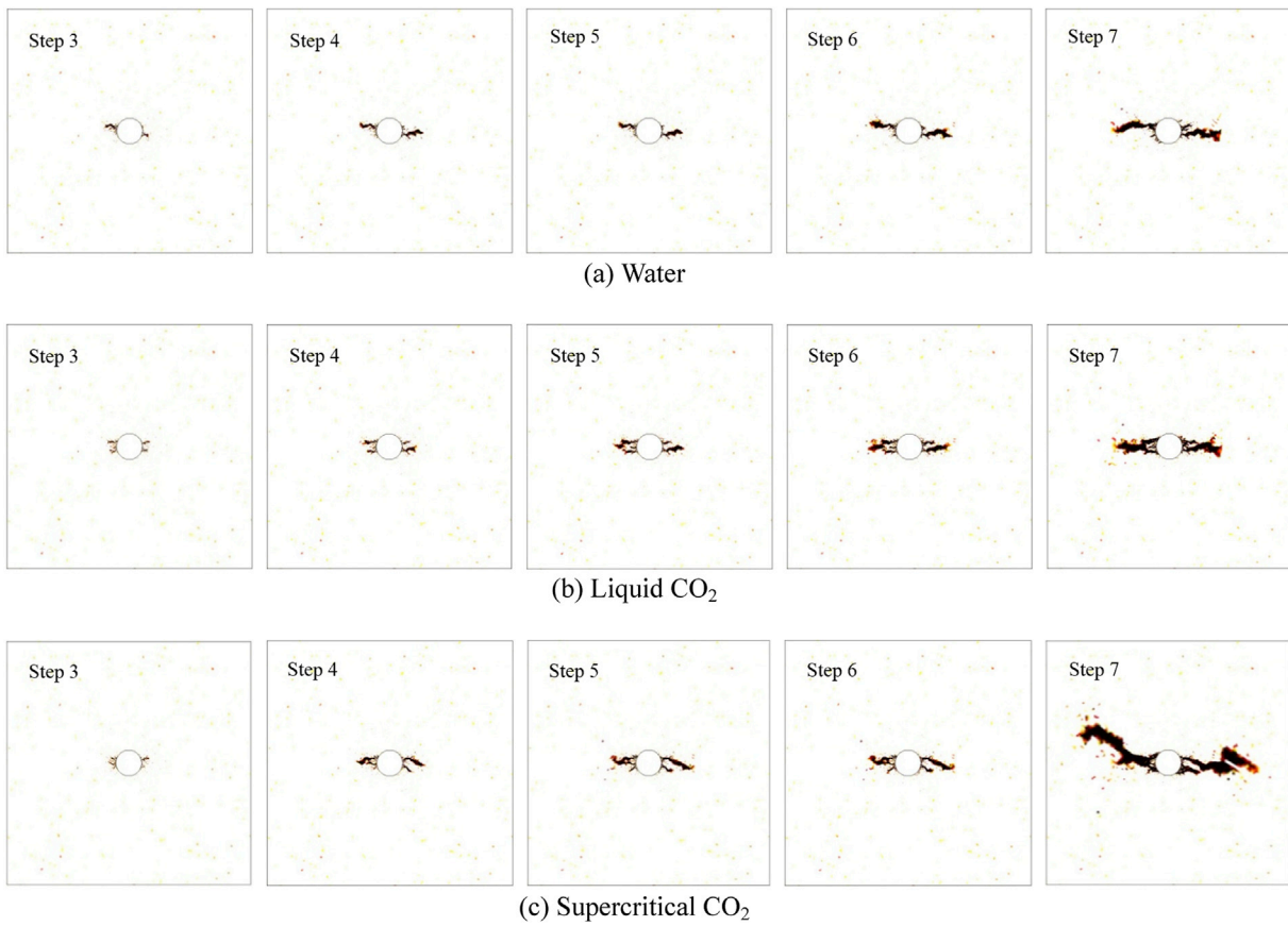
Fig. 14. Fracturing patterns under different injected fluids when lateral pressure coefficient \lambda = 2 .
