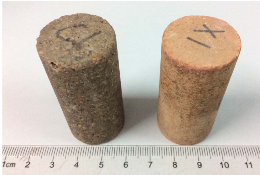
Figure 1. Specimens investigated in the imbibition tests. C1 is a coarse-grained sandstone, and X1 is a silty sandstone.
