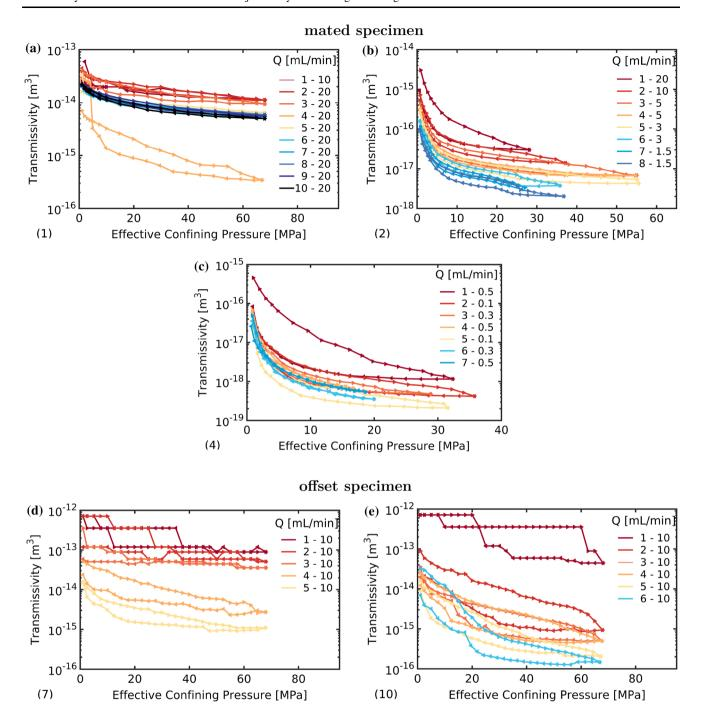
Fig. 4 Tests 1, 2, 4, 7 and 10 are shown in subfigures a-e, respectively. The plots show transmissivity (Eq. 4) versus effective confining pressure. The first number in each row in the legend denotes the cycle number, with *color coding* of the data curves going from the first cycle (*dark red*) to the last cycle (*dark blue*). The second number
