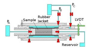
**Fig. 2** Experimental setup of core holder and specimen. The pressures were prescribed in pumps  $P_A$  (axial pressure  $p_{ax}$ ),  $P_B$  (confining pressure  $P_{co}$ ) and  $P_C$  (fluid inlet pressure  $p_{fp}$ )
