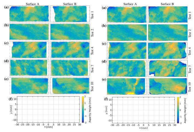
**Fig. 8** Surface scans before testing. Specimens from tests 1, 2, 4, 7 and 10 (*top to bottom*, **a–e**) with surfaces A (*left*) and B right before testing. A reference figure for the surface scan dimensions and asperity height *colorbar* is shown in **f** (color figure online)
