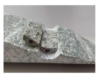
Fig. 1 Example of overcored specimen on top of one fracture surface
