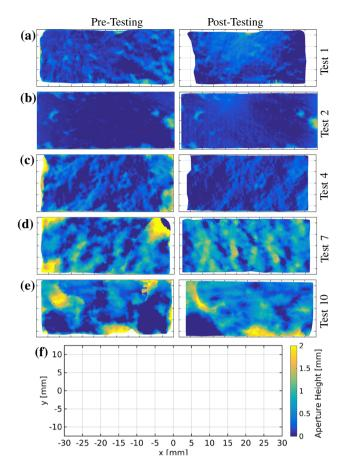
**Fig. 10** Aperture fields as derived from surface scans (Figs. 8, 9). Specimens from tests 1, 2, 4, 7 and 10 ( $top\ to\ bottom$ ) with apertures before (left) and after (right) testing. Reference figure for the aperture field dimensions and aperture size colorbar is shown in  $\mathbf{f}$  (color figure online)
