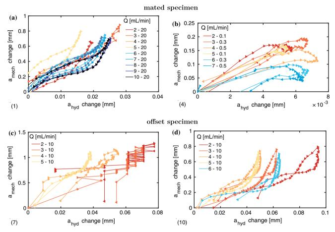
**Fig. 5** Mechanical versus hydraulic aperture changes. Changes are calculated by comparison with the initial values at 1 MPa. Specimens from tests 1, 4, 7 and 10 are assigned to **a–d**, respectively. The curve
